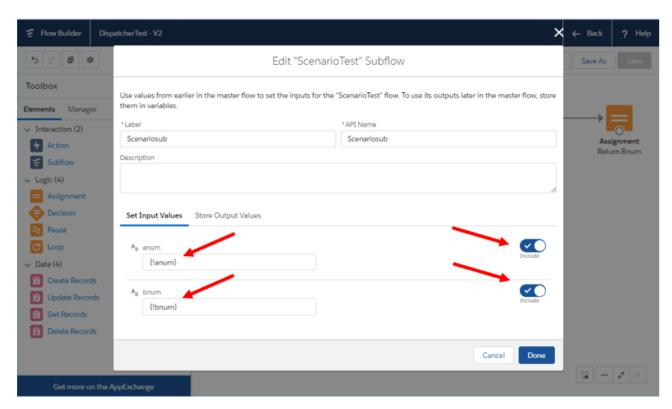
Check 'Manually assign vabiables (advanced) and the following components must also be set under 'Store Output Values'; allocationTargets, FailTarget, InitialTarget, Priority and RequiredTarget. (anum and bnum are left empty here)
