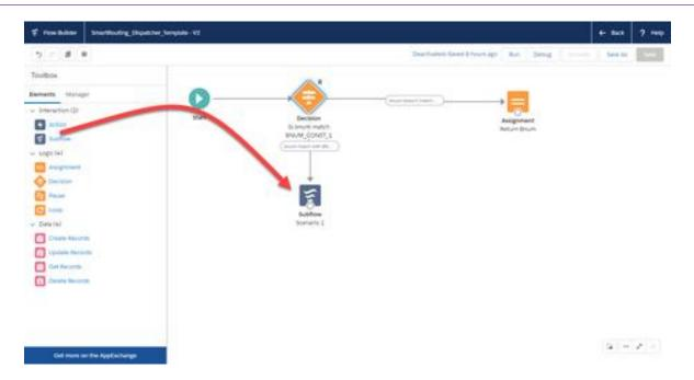
Components anum and bnum must be set and included under '**Set Input Values**' while setting the subflow.
