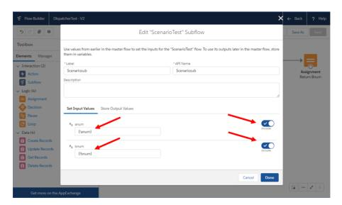
The following components must also be set under '**Store Output Values**'; allocationTargets , FailTarget, InitialTarget, Priority and RequiredTarget. (anum and bnum are left empty here)
